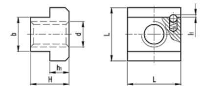
b -0.1 -0.3 = 12 d = M10 H = 14 h1 = 7 L = 18 I1 = 0.7 T-slot width DIN 650 = 12 Weight (g) = 22
